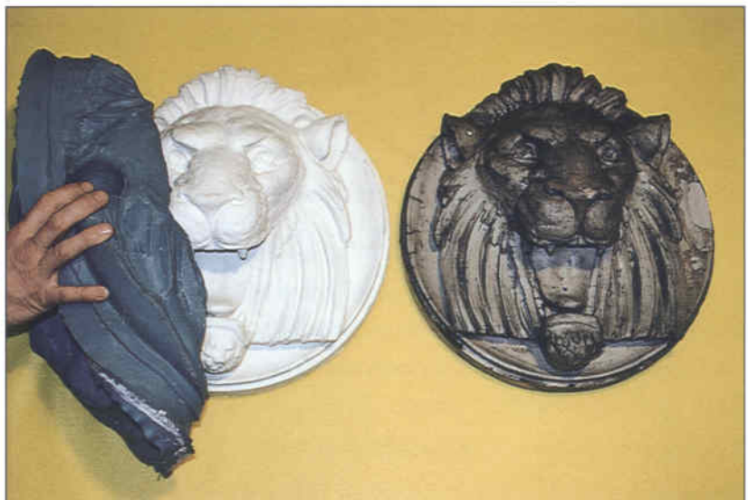
In the picture above the MasterMold 12-3 is removed from a casting of the terra cotta lion's head.
